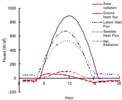
Figure 3a. Energy balance in unirrigated condition
