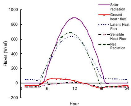
Figure 3b. Energy balance in irrigated condition
