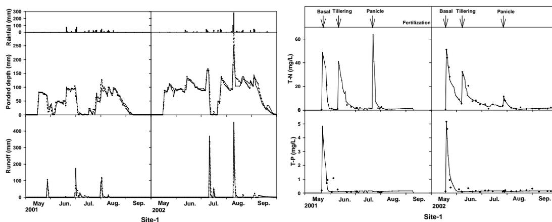
Fig. 1. Observed and predicted nutrient concentrations of ponded water and surface runoff in the paddy rice fields
