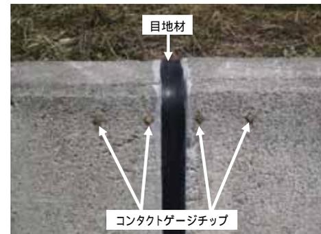
Fig.3 Position of contact gauge chip
