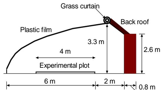
Fig.2 Vertical cross-section of Chinese style greenhouse
