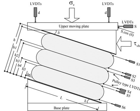
Fig. 2: Specimen with bedding planes at an angle of 18 degrees relative to the horizontal set in a lateral shearing apparatus.
