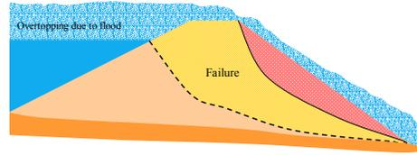
Fig. 1: Typical failure modes of small earth dams.
