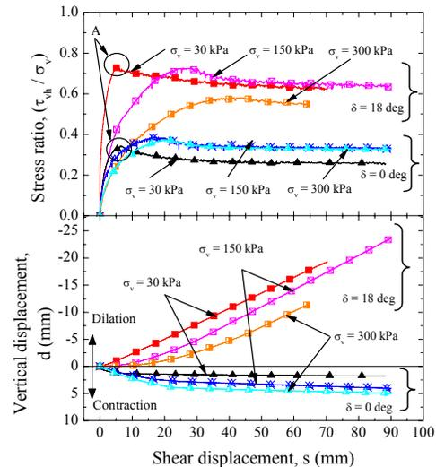
Fig. 3: Relationship among stress ratio, shear displacement and vertical displacement from tests at different  $\sigma_v$  values at  $\delta = 0$  & 18 degrees.
