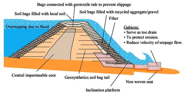
Fig. 5: Earth dam with inclined soil bags having a geotextile tale constructed by a newly proposed technology.
