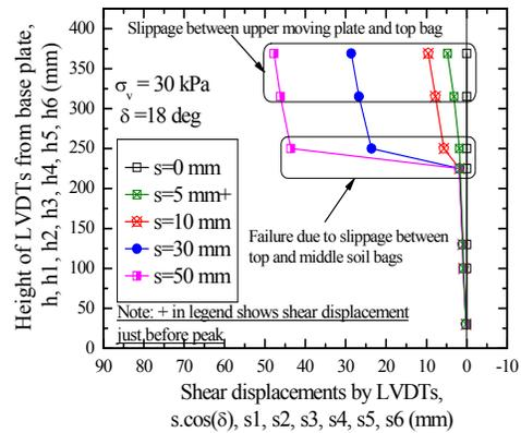
Fig. 4a: Distribution of lateral displacement of soil bags along height, at a low normal stress.
