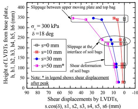
Fig. 4b: Distribution of lateral displacements of soil bags along height, at a high normal stress.
