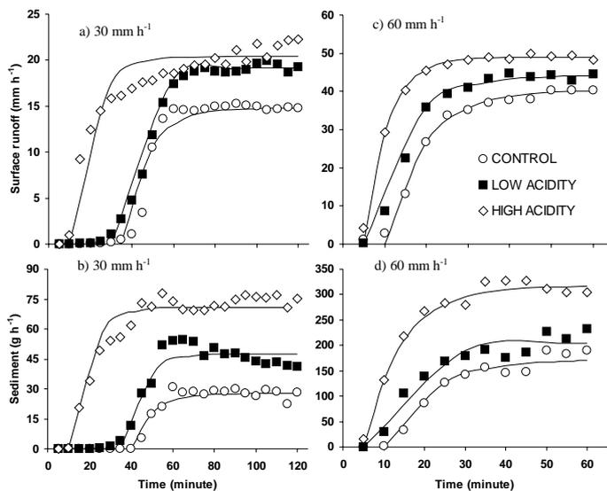
Fig. 1 The three phase temporal changes in surface runoff and sediment generation.
