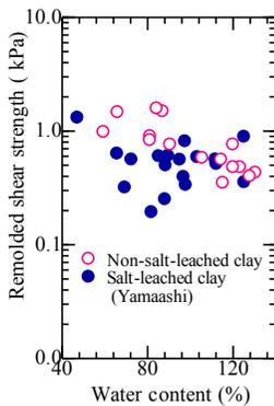
**Fig.4. Remolded shear strength versus natural water content for salt-leached and non-salt leached clay**
