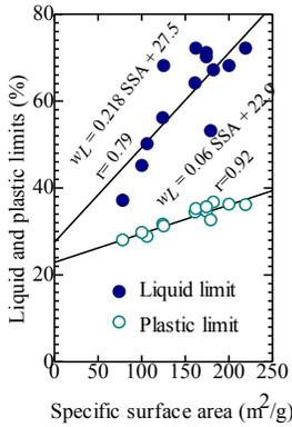
**Fig.3. Relationship between consistency limits and specific surface area**
