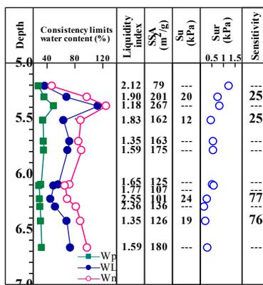
Fig.2. Geotechnical properties clay profile at Yamaashi
