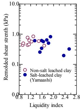
**Fig.5. Remolded shear strength versus liquidity index for salt-leached and non-salt leached clay**
