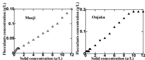
Fig. 3. Relation between solid concentrations versus polyaluminium chloride flocculant (PAC) concentration needed for the flocculation of soil suspensions.
