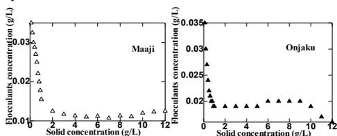
Fig. 4. Relation between the solid concentrations versus polyaluminium chloride flocculant (PAC) per unit soil weight for the flocculation of soil suspensions.
