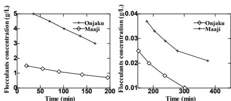
Fig. 5. Time for setting of flocculants at different flocculant concentration.
