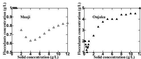
Fig. 2. Relation between solid concentrations versus volcanic ash soil flocculant (VAS) per unit soil weight for the flocculation of soil suspensions.
