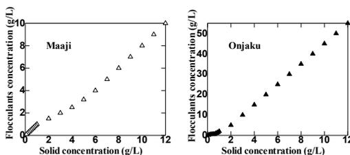
Fig. 1. Relation between the solid concentration and the volcanic ash soil flocculant (VAS) concentration needed for flocculation of soil suspensions.
