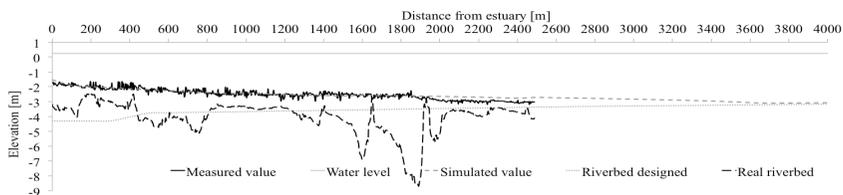
(b) The observed and simulated salt water wedge for a neap tide
