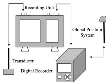
Figure 2 Acoustic profiling system
