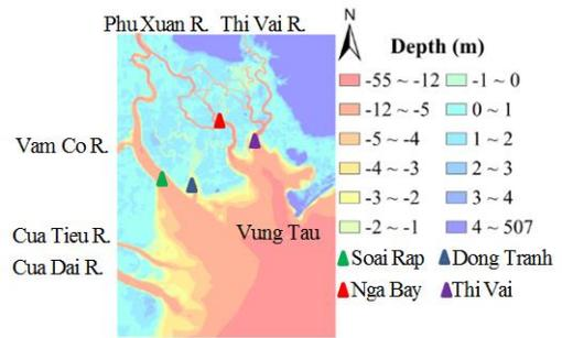
**Figure 1. Bathymetry and model domain in the Can Gio Bay**
