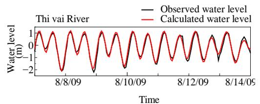
**Figure 2. Observed and calculated water level of the Thivai River from 00:00 (GMT+7) August 7 to 00:00 (GMT+7) August 14, 2009**
