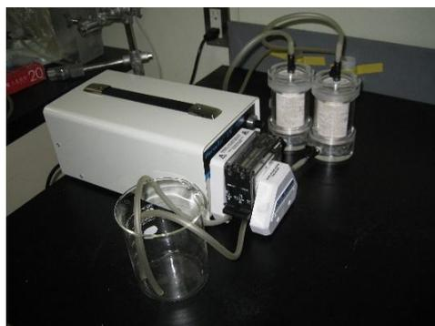
Photo.1 Column test for curing
