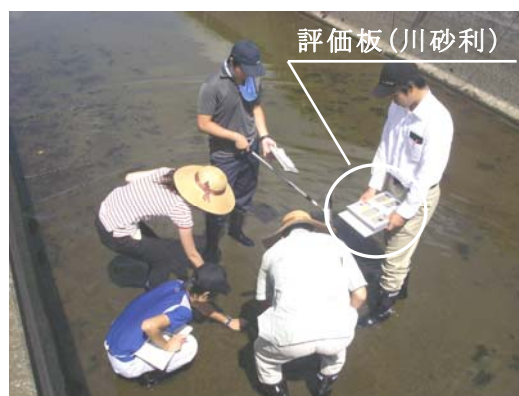
図-1 評価板法による粗度係数推定状況 Estimation of Manning's roughness coefficient in the existing concrete open channel
