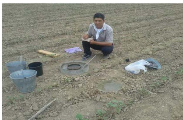
Fig. 2. Measurement of water permeability
