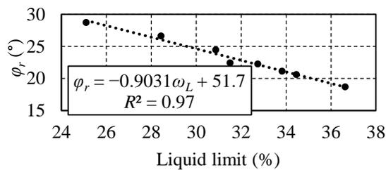
Fig. 1 Residual frictional angle vs. liquid limit (Fang *et al.*, 2019)
