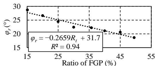
Fig. 3 Residual frictional angle vs. ratio of FGP
