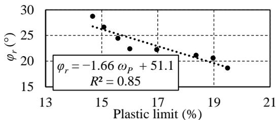
Fig. 2 Residual frictional angle vs. plastic limit (Fang *et al.*, 2019)
