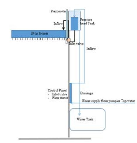
**Fig. 1** Diagram of the Mini Portable Pressure Head type rainfall simulator (MPPH)
