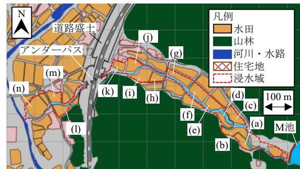
Fig. 1 M池氾濫域の概要 Inundation area due to M-dam breach
