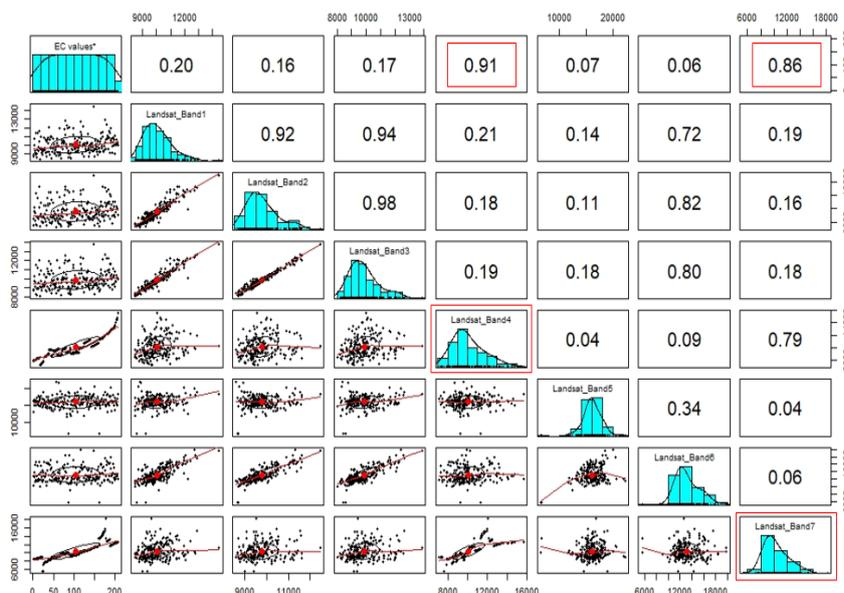
**Fig.2** Pairs and panels statistical output for the EC values and Landsat
