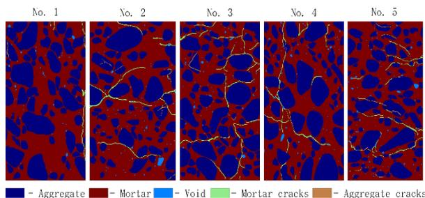
Figure 1. Internal cracking system
