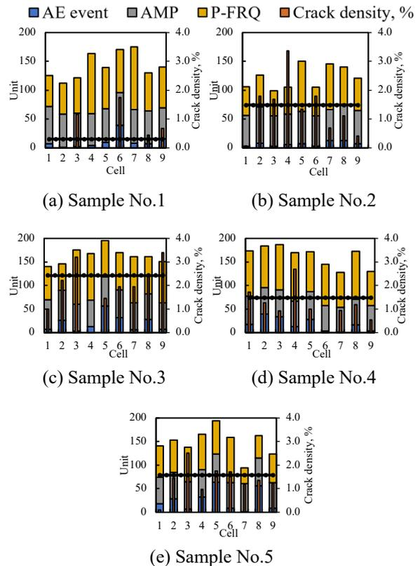
Figure 2. Relationship between cracks and AE signal parameters
