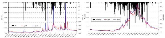
Fig.4 Observed and calculated hydrographs at Stoeng Treng (T-2) and at Kontum (T-5)
