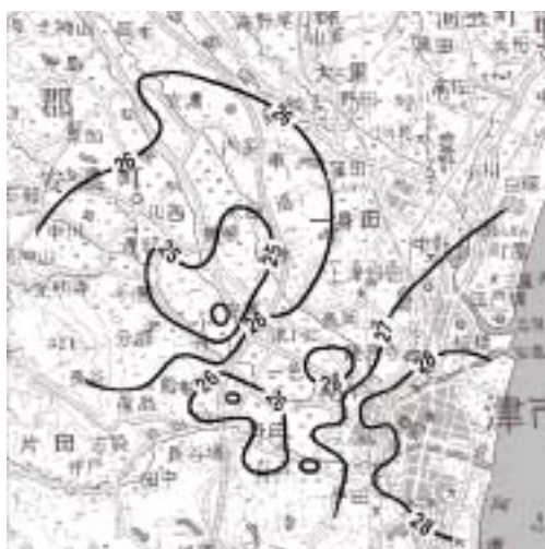
Fig.1: Temperature distribution in the Anou River Basin at night on July 26, 2001
