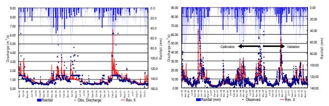
Fig. 4 Performance of Rev. II at Cikalumpang Weir
