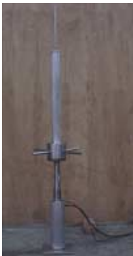
Fig-1 Waterway penetro-meter
