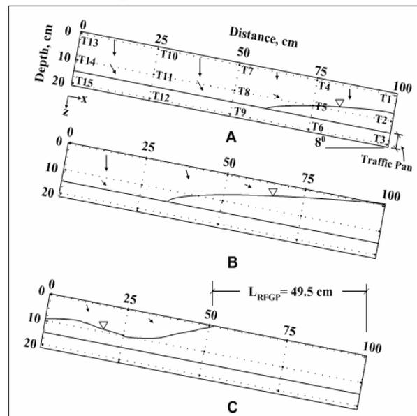
Fig. 3 Illustration of water table position and flux distributions at different times of the experimental run 2: (A) at elapsed time  $t = 180$  min, maximum flux velocity is 0.192 cmh<sup>-1</sup>; (B) at  $t = 360$  min, maximum flux velocity is 0.15 cmh<sup>-1</sup>; and (C) at  $t = 600$  min, steady state is attained, maximum flux velocity is 0.07 cmh<sup>-1</sup>, RFGP is observed at 49.5 cm from the downslope end, which is considered to be at the midslope.
