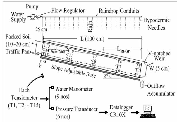
**Fig. 1 Generalized schematic of laboratory setup and definition sketch of RFGP.**
