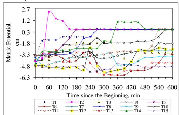
Fig. 2 Matric potentials in the model slope for the experimental run 2. Here, observation nodes T1, T2, etc. are shown in Figures 1 and 3.
