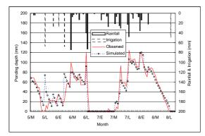
Fig. 1. Comparison of measured and predicted daily ponding depth
