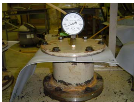
Fig.2 Water pressure resistance test
