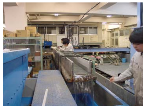
Fig.3 Measurement of coefficient of roughness
