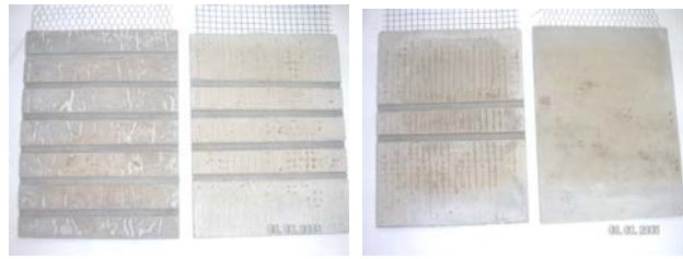
Fig. 5 Ferrocement with smooth and rough surfaces
