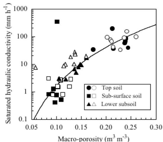
**Figure 3.** Saturated hydraulic conductivity as a function of macro-porosity. Closed and open symbols represent Gamba grass and Stylo, respectively.
