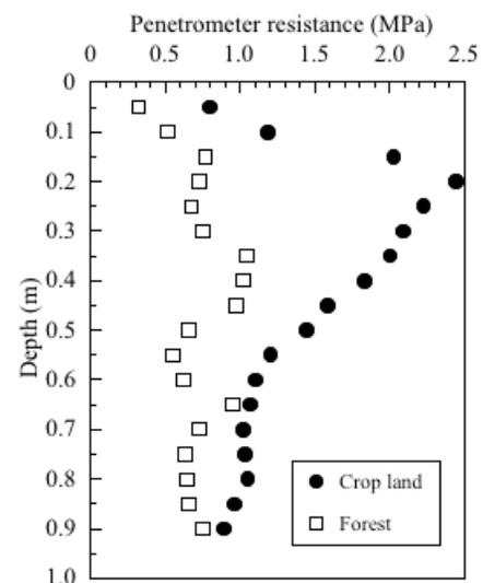
**Figure 1.** Effect of changed land use on penetrometer resistance in Northeast Thailand.
