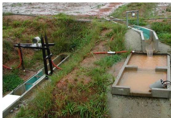
Fig.3 Observation equipment of discharge and turbidity
