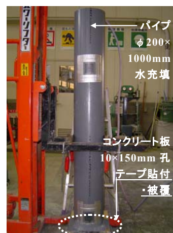
Fig.4 Water leak amount test
