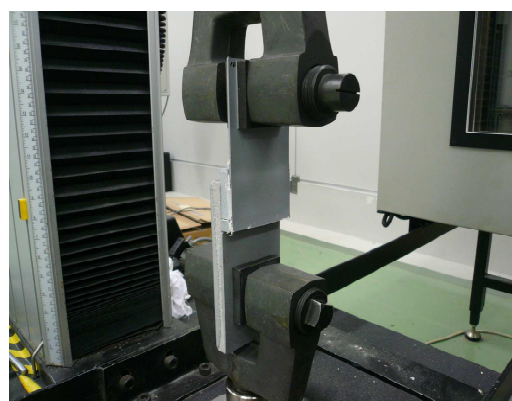
Fig.5 Tensile characteristic test
