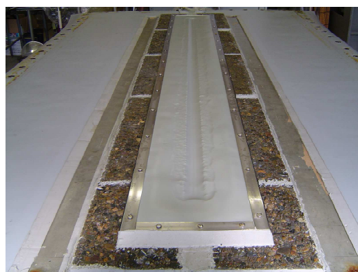
Fig.4 Result of water pressure resistance test
