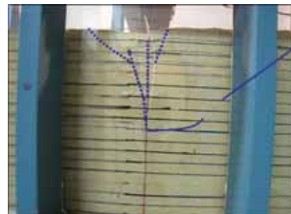
Fig.4 Deformation around the wall after peak vertical load
