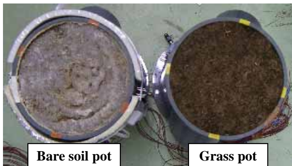
Fig.3 Photo of soil surface of salt-supplied pots after 35 days of salt water supply. Soil surface of the grass pot was exposed by cutting grass. Salt precipitate was observed in the bare soil pot, but that was not observed in the soil surface of the grass pot.
