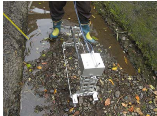
Fig.6 携帯型凹凸測定器による水路形状の調査 Investigation of irrigation canal shape with portable ruggedness measure
