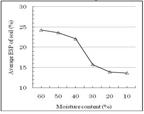
Fig. 3 The average ESP of soil against various initial water contents.
