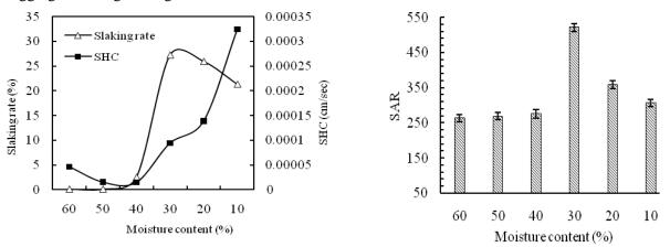
**Fig. 1** Saturated hydraulic conductivity (SHC) and slaking rate of soil to moisture content.
