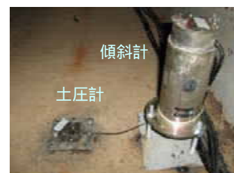
図-3 土圧計と傾斜計の設置 Earth Pressure Gauge and Clinometer
