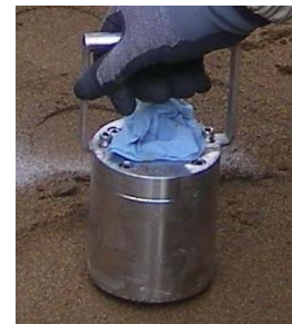
図1 ソイルテスト Soil stiffness measuring device (Soil Test)
