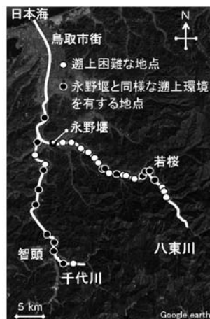
Fig.1 堰堤・魚道の現状 Condition of weirs and fishways in the Sendai River system
