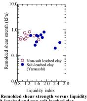
Fig.5. Remolded shear strength versus liquidity index for salt-leached and non-salt leached clay
