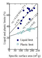
Fig.3. Relationship between consistency limits and specific surface area
