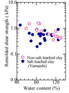
Fig.4. Remolded shear strength versus natural water content for salt-leached and non-salt leached clay
