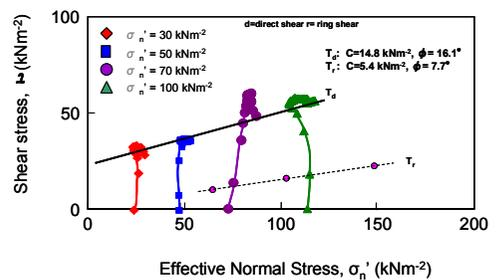
Fig.2. Stress paths and stress envelopes for Tyunjun sample within ENS range of 30-150 kNm<sup>-2</sup> in direct and ring shear tests
