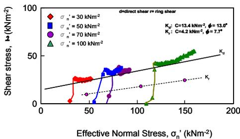
Fig.1. Stress paths and stress envelopes for Kamenose sample within ENS range of 30-150 kNm<sup>-2</sup> in direct and ring shear tests
