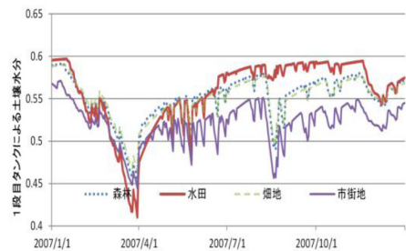
Fig.5 土壌水分量の計算結果 (サブ流域 25) Calculated volumetric water content ratio (Sub watershed No.25)
