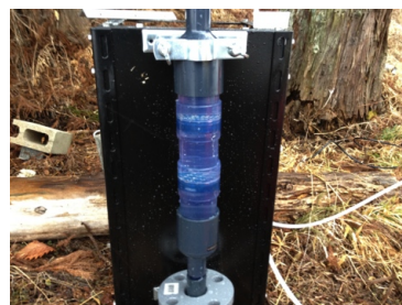
Fig.1 吸引法の実施状況 Cs monitoring system using PB nonwoven fabric (Suction type)
