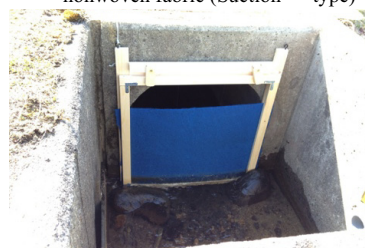
Fig.2 固定法の実施状況 Cs monitoring system using PB nonwoven fabric (Fixed type)
