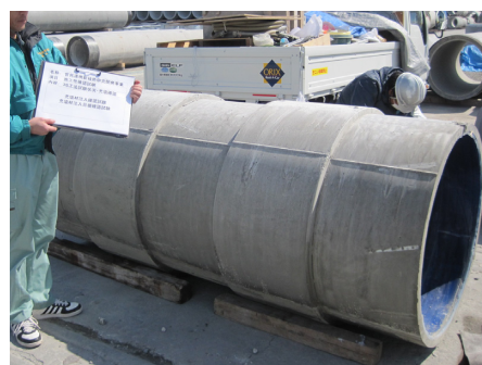
Pic 2 模擬管路脱形状況 The situation dismantled formwork
