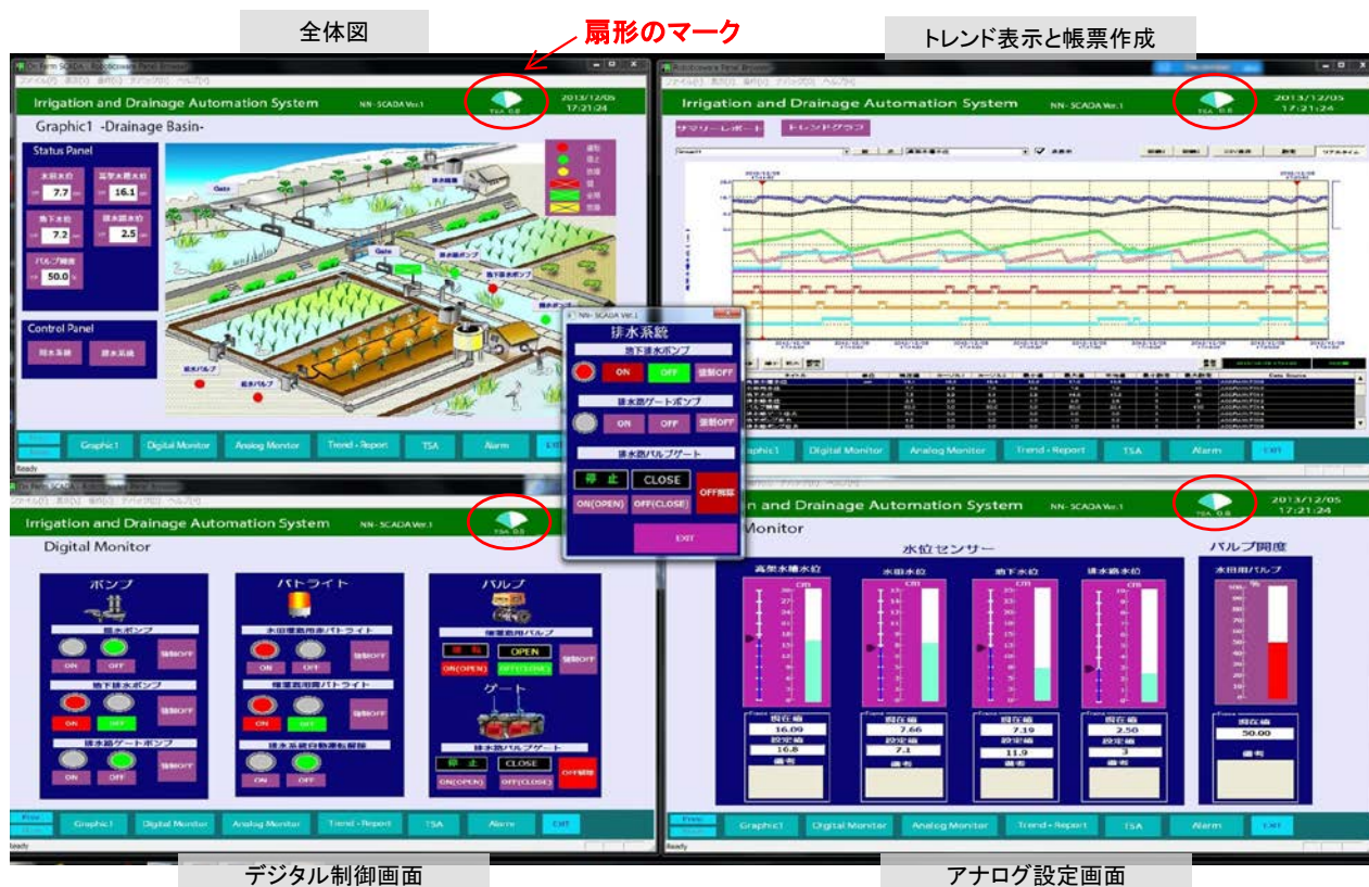
図3 SCADA上の監視制御画面 Supervisory control monitor on SCADA
