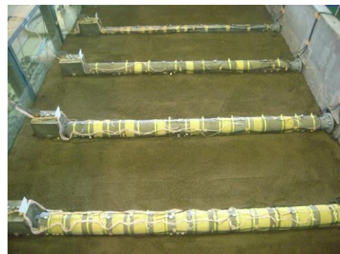
Fig. 1 模型管設置図 Model pipes during back-filling
