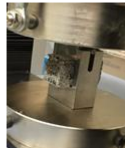
Fig. 1 圧縮試験治具，供試体 Unconfined compression specimen and fixture
