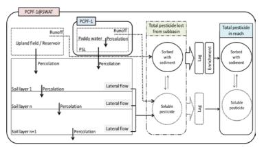
Figure 1. Water and pesticide routing from rice paddy in the PCPF-1@SWAT model (Boulange, Watanabe et al. 2014).
