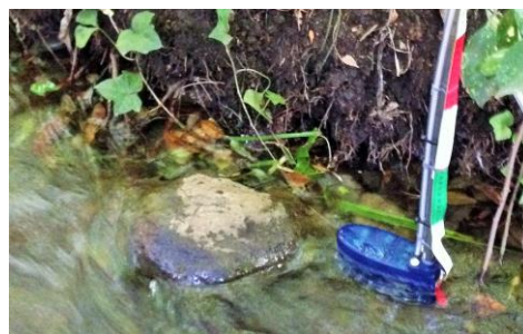
Fig. 1 An artificial lateral line probe for high frequency flow measurement
