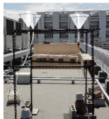
Photo 1 Rainwater sampler
