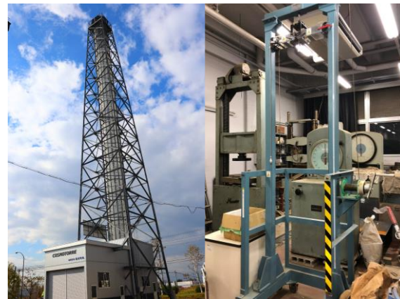
図1. 50 m 落下塔 (左) と 2 m 落下施設 (右) Figure 1. 50 m Drop tower(left) and 2 m Drop tower(right).
